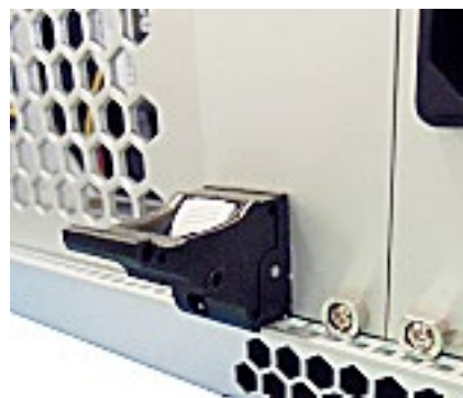
Fig. 82 Pull-out lever of the power supply unit of chassis 474-BODY21/4U
