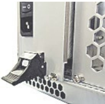
Fig. 82 Pull-out lever of the power supply unit of chassis 474-BODY21/4U
