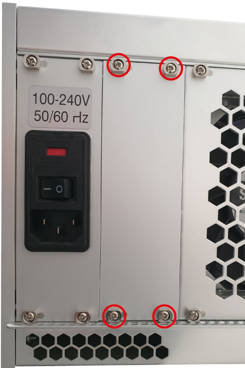
Fig. 81 Removing the blanking plate from chassis 474-BODY21/4U
